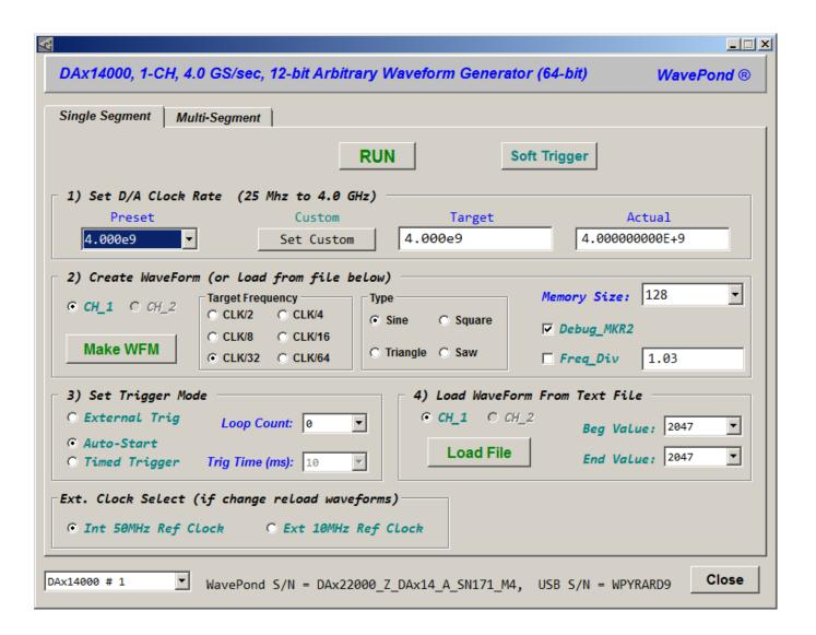
Use "dax14000\_GUI\_xx.exe" GUI to verify drivers are installed correctly and to load simple sine and custom waveforms. (xx = 32 or 64)
